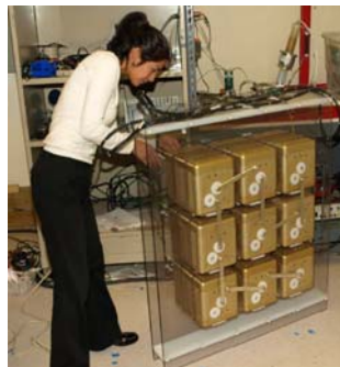
Fig. 2. Nine cells of the short-pulse Marx mounted in a rack for system testing.
